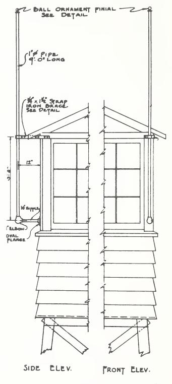
Figure 66. R-6 design for 7 feet square wooden cab for use with 100 feet and 120 feet high timber towers. This detail from the 1934 plans illustrated placement of the flagpole.
